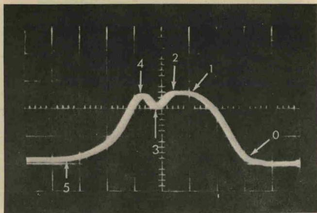
FIG. 4. Oscilloscope record of the induced positive voltage in a silicon crystal when stressed initially to 12 kbar. A second shock enters the crystal from the shock-driving system at  $\sim 0.4 \mu\text{sec}$  after the 12-kbar shock entered. This second shock takes the crystal to a stress of  $\sim 90$  kbar. No voltage was applied to the crystal. Time increases from right to left. The vertical scale is 1.0 V/div and the horizontal scale is 0.11  $\mu\text{sec}/\text{div}$ .
