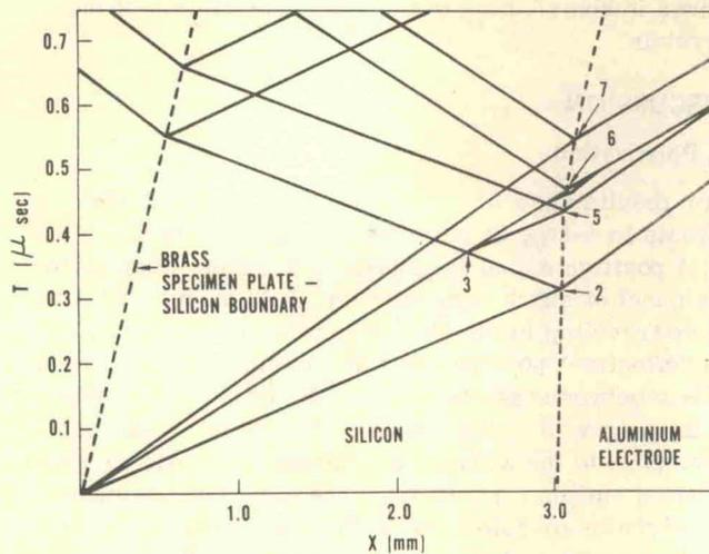
FIG. 2.  $x-t$  diagram of shock-wave propagation in silicon for the experimental arrangement of Fig. 1. The stresses behind the three forward-facing shock waves are 55, 133, and 162 kbar, respectively.
